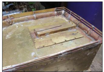
Photo 11 shows all the coal rails and backing plates place and soldered into position. There aren't backing plates at the back so the coal rails can be seen more clearly there. There is still a bit of cleaning up to do. but at least I have now completed coal rails the assembly.
