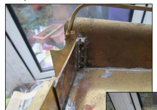
When I started out the only screws I had were a bit long! **Photo 8** shows the upper coal rail being attached.
